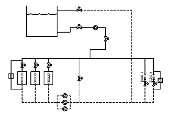
When the tank is brought on line, the appropriate control valves are position to allow the tank pumps to deliver chilled water into the supply line, and have the building return water be dumped into the top of the tank. During this mode of operation, the operating chiller(s) are run at rated design flow. The tank pumps are operated to provide enough chilled water required by the system which cannot be produced through the chillers.
