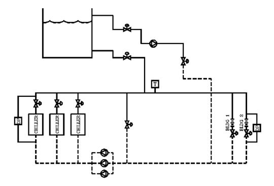
During the evening hours, once the load in the system begins to back off, the excess chilled water available is sent to the tank. The tank valves are positioned to allow the chilled water to go into the bottom of the tank, and the warm tank water to be drawn from the top of the tank.
