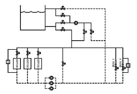
The new chiller plant distribution system is a Systecon VariPrime chilled water pumping system, and the tank system is a standard Systecon variable speed pumping system. The VariPrime system allows for variable flow through the evaporators to account for the different return temperatures coming from the buildings and the tank. The tank pumps are sized to pump the entire system when chilled water is required from the tank.
